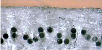
**MicroPrexx™** combines ultra-high density with compression controlled batt for high nip dewatering efficiency. The high fibres diameter, plus the ultra-high density Polyamide 6.0 developed, ensures the best elastic response, thus resistance to chemical degradation by a permanent self-washing of the felt in the nip.
