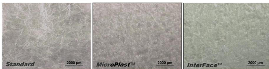
**MicroPrexx™** benefits from **InterFace™**, special anti-pilling polymeric surface layer. This innovative solution offers a dense surface, very regular and free of fibres pilling. When Bendtsen, two-sidedness, even coating are issues, **InterFace™** is a key.
