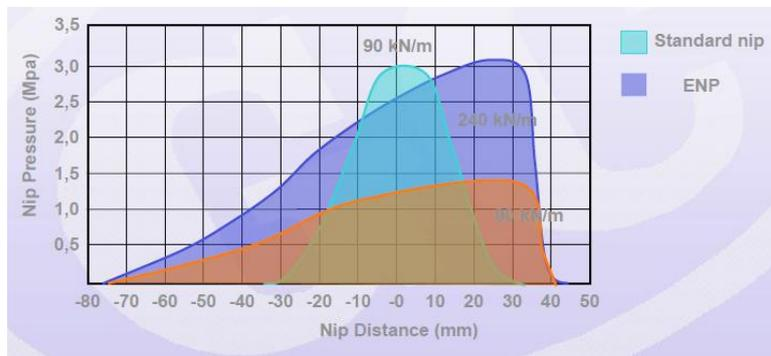
The high compressibility of **MicroPrexx™** allows a low thickness (faster water flows transfers) felt under the higher pressure in the first part of the nip for an efficient dewatering; when its elasticity recovers full thickness in the depressed end of the nip, slowing down flow transfers, thus rewetting. In addition the **InterFace™** layer contributes to strongly break down the possible rewetting water.
